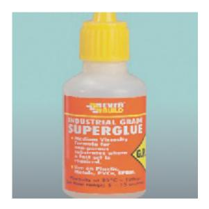
Medium viscosity formula fills gaps to 0.1mm. For use on perfect fit surfaces where fast set is required. Bonds non porous surfaces eg most plastics, metals, glass, PVCu, rubber and EPDM. Viscosity at 25°c - 100cps. Set time 5 to 15 seconds.
