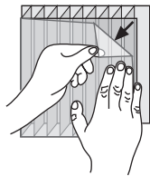
Figure 17a. Partial or Complete Removal of Protective Foil Prior and after Installation
